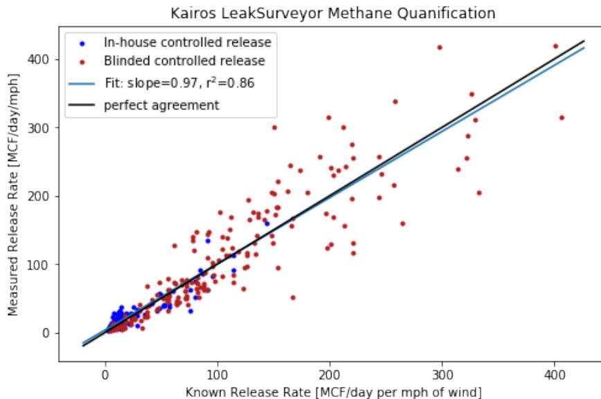
Figure 4: Quantification of methane release rate shown for controlled release data from nine different occasions in three different locations and on three different instruments. The best fit line shows excellent agreement with the line of perfect agreement.
