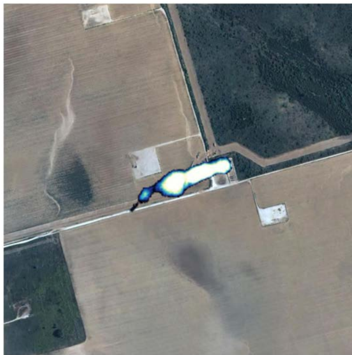
Figure 1—Example of plume detection. A methane plume image, colored by methane concentration from blue (low) to white (high), generated by the imaging spectrometer, is seen to emanate from a well pad that was imaged using the high-resolution optical camera.
